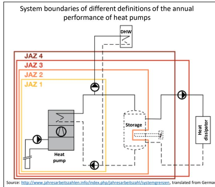
Figure 2. System boundaries of different definitions for the annual efficiency of heat pumps
