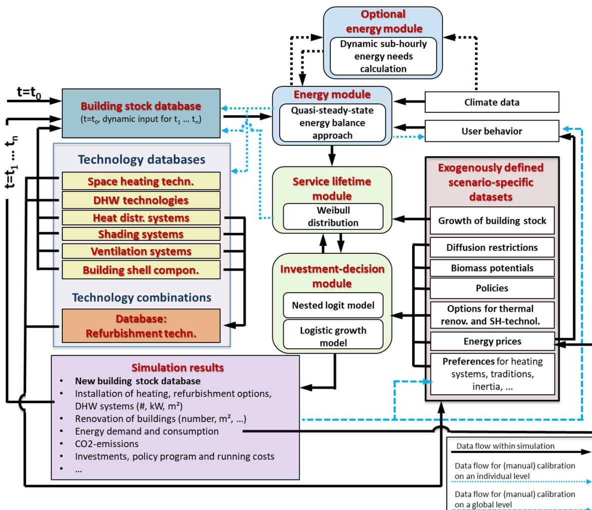
Figure 1: Overview of the structure of Invert when applying the EE-Lab version
